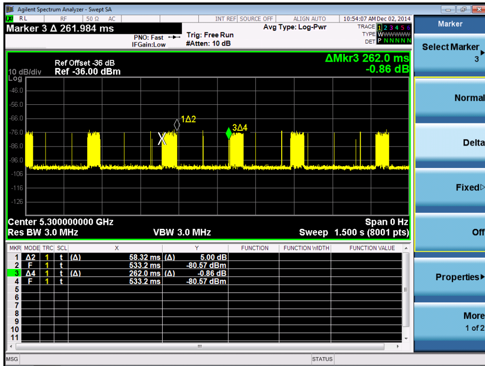
Channel Loading Plot - 802.11n-HT20 - 5300MHz
