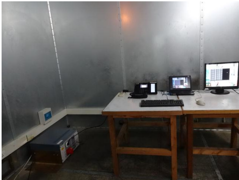
Conducted Emission Test Set-up -Front View
