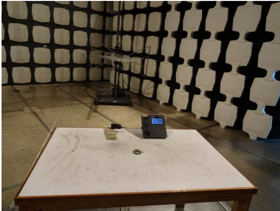
Radiated Emission Test Set-up -below 1GHz
