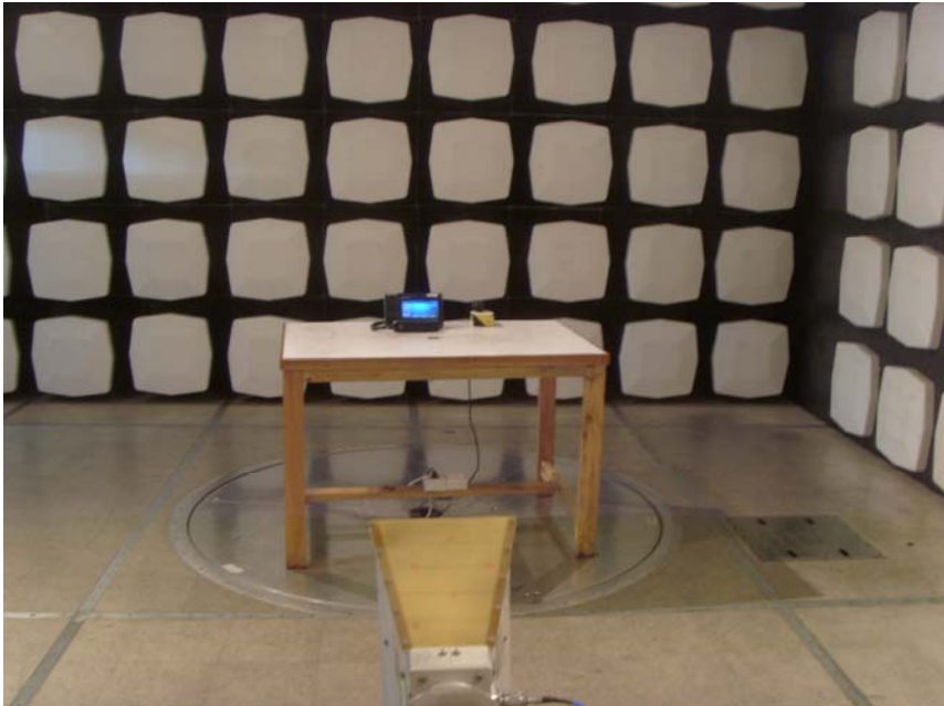
Radiated Emission Test Set-up – Above 1GHz
