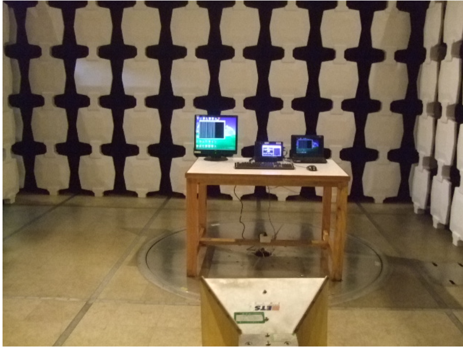
Radiated Emission Test Set-up - Above 1GHz
