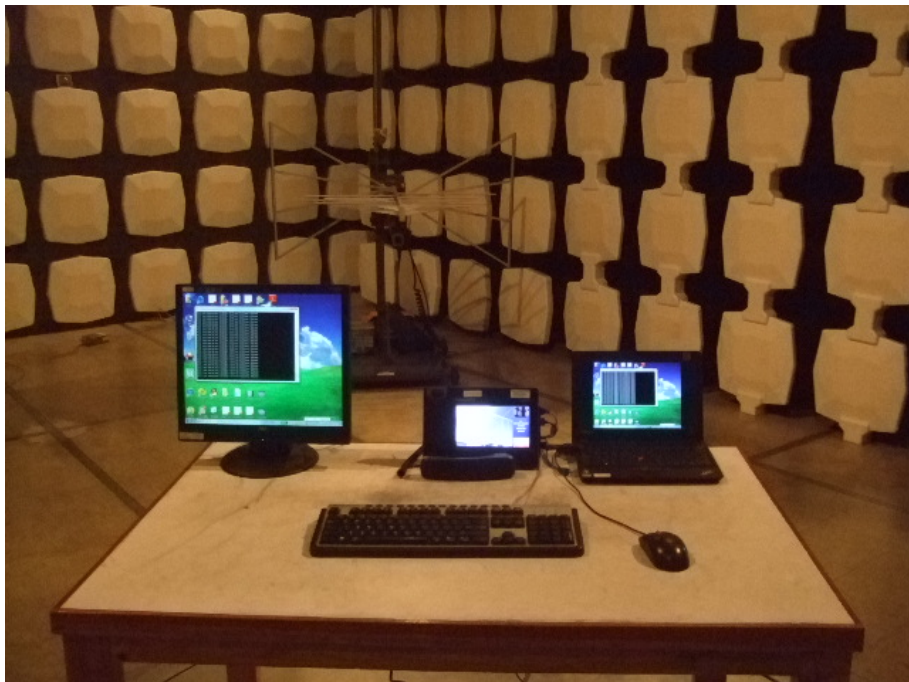
Radiated Emission Test Set-up -below 1GHz
