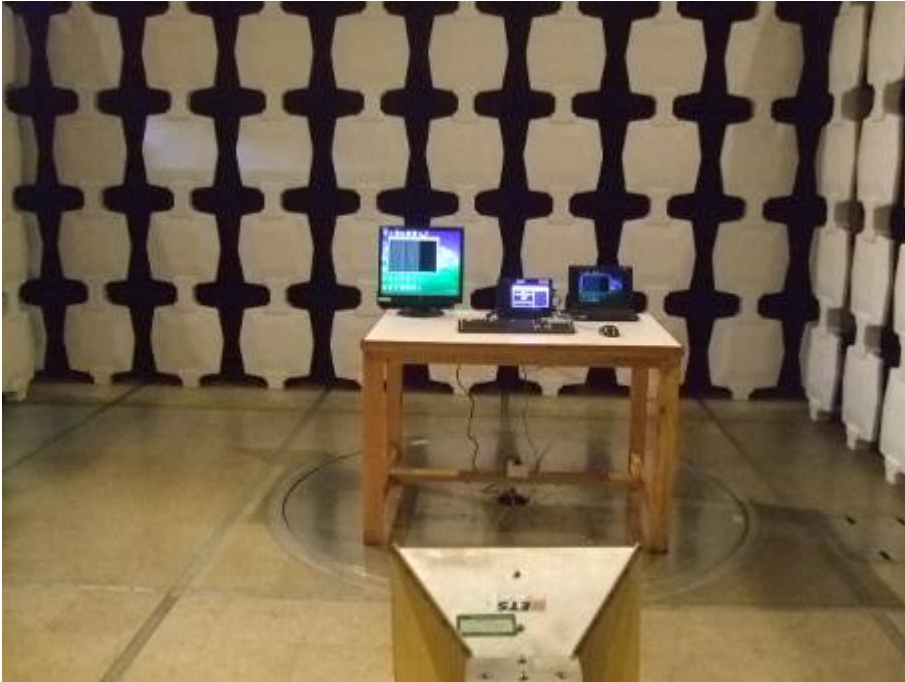
Radiated Emission Test Set-up - Above 1GHz
