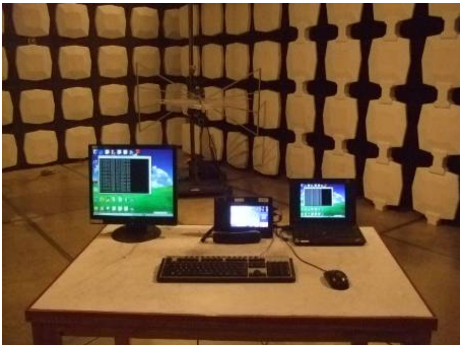
Radiated Emission Test Set-up -below 1GHz
