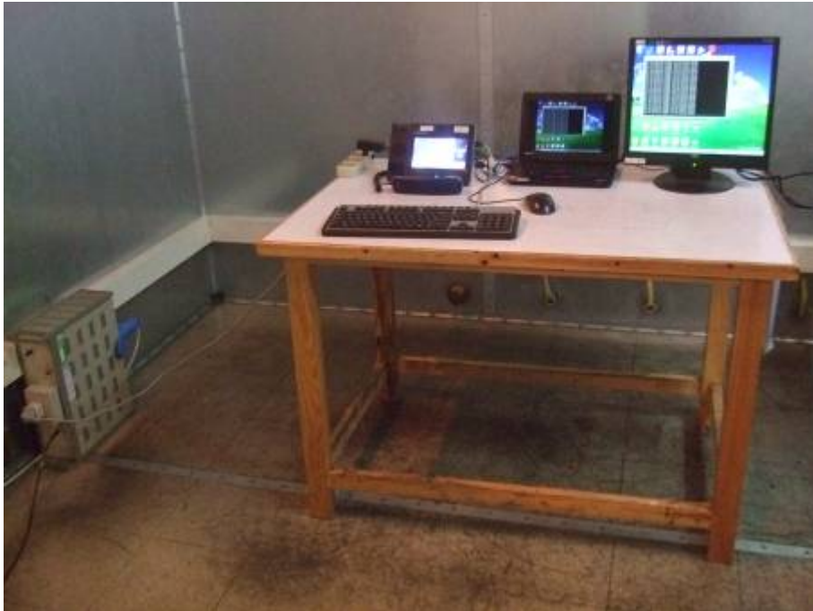
Conducted Emission Test Set-up
