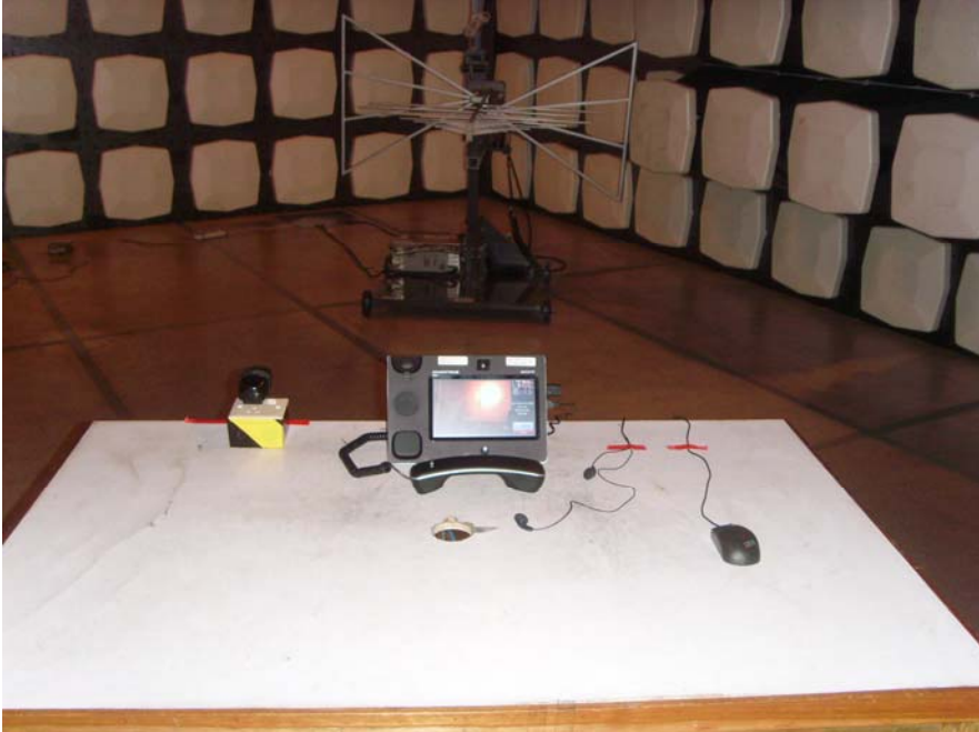
Radiated Emission Test Set-up(Below 1GHz)
