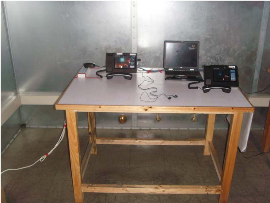
Conducted Emission Test Set-up
