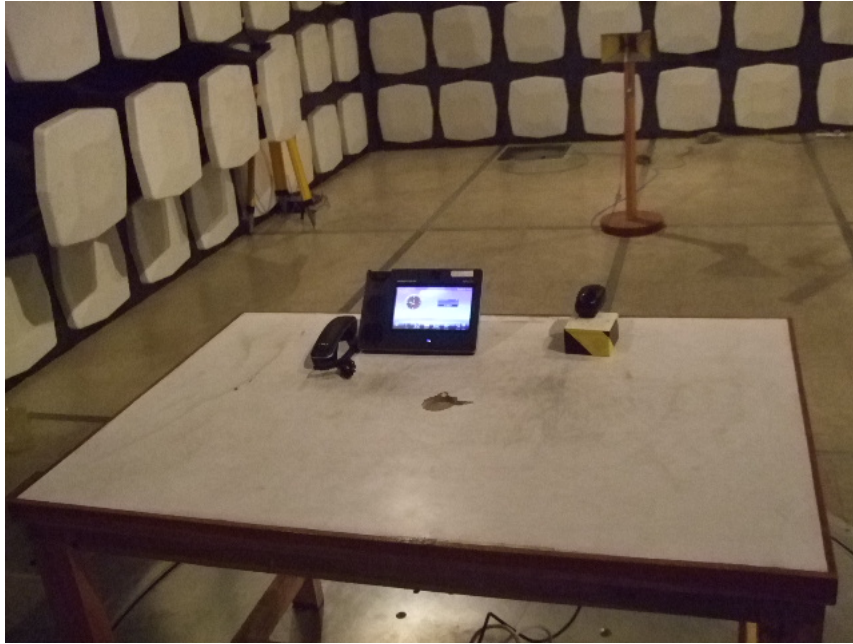
Radiated Emission Test Set-up - Above 1
