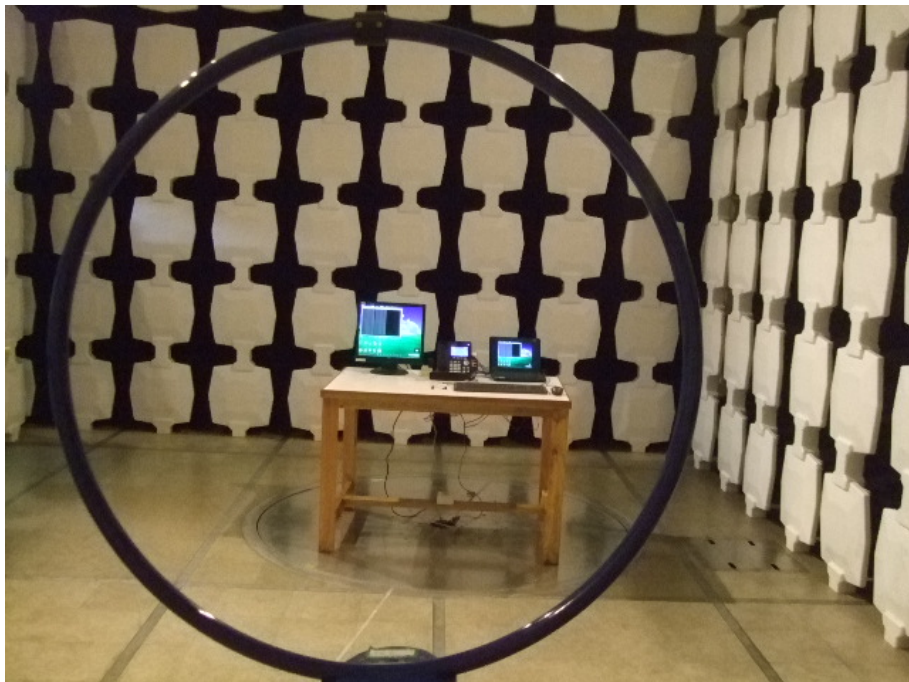
Radiated Emission Test Set-up (9KHz-30MHz)
