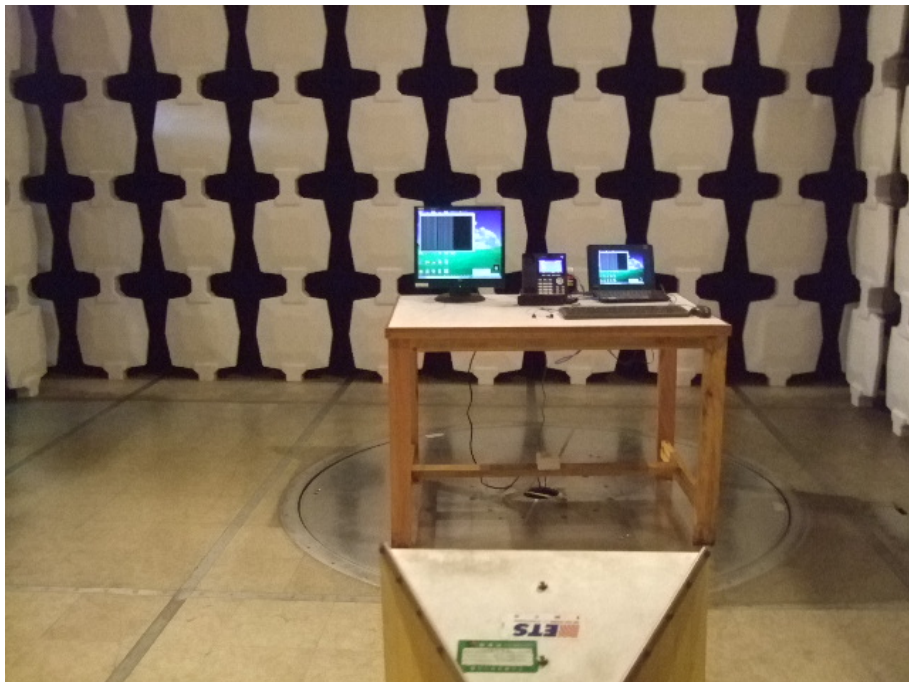
Radiated Emission Test Set-up (Above 1GHz)
