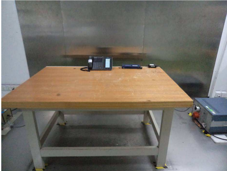
Conducted Emissions - Front View (Powered by PoE)
