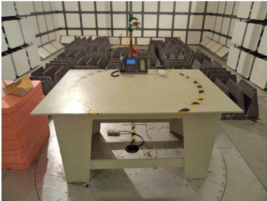
Radiated Emissions – Front View (Above 1 GHz)
