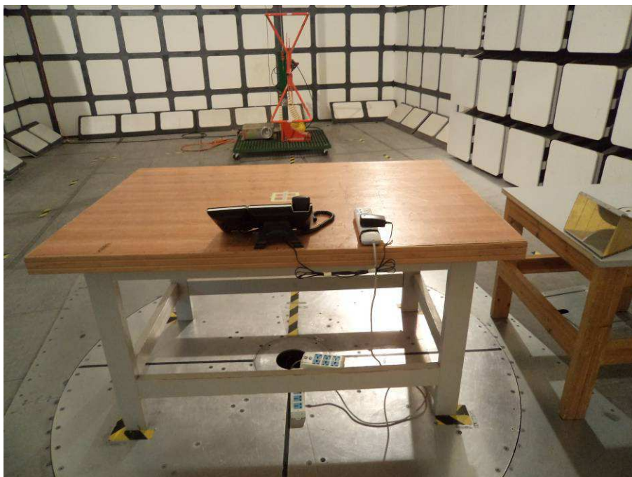
Radiated Emissions – Rear View (Below 1 GHz)
