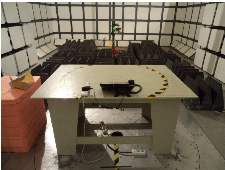
Radiated Emissions – Rear View (Above 1 GHz)
