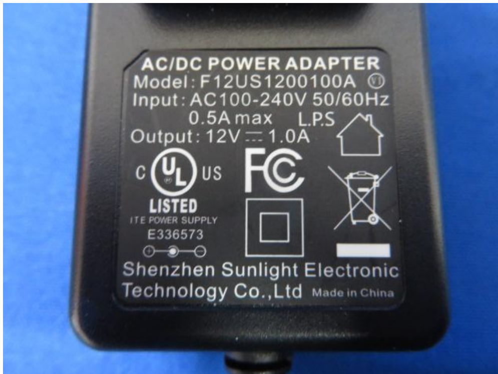
(22) EUT Photo (Adapter #1)
