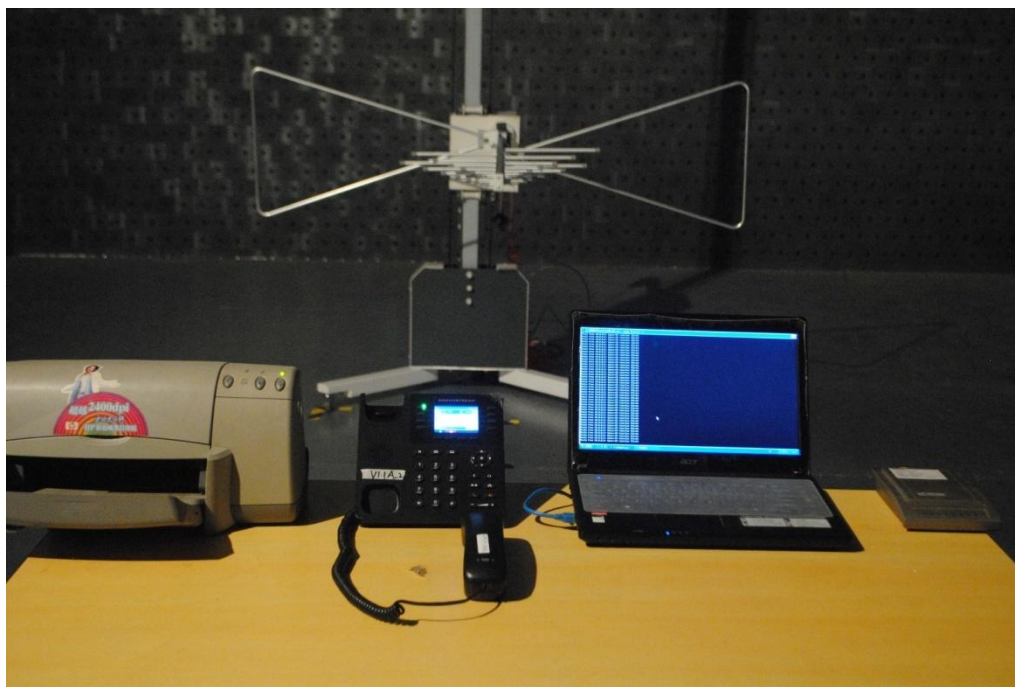
Radiated Emission test view (Frequency above 1GHz)
