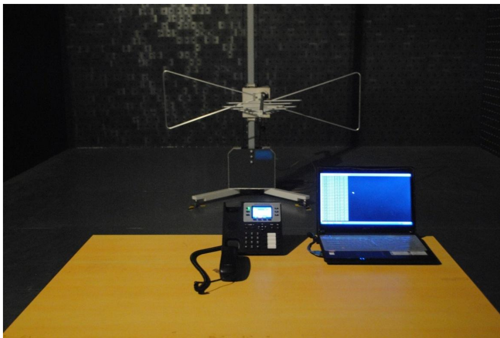
Radiated Emission test view (Frequency above 1GHz)
