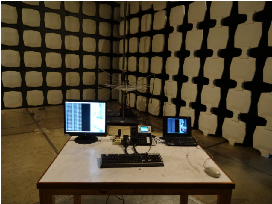
Radiated Emission Test Set-up (Below 1GHz)
