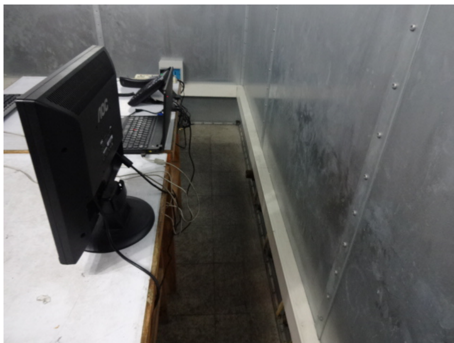
Conducted Emission Test Set-up -Rear View
