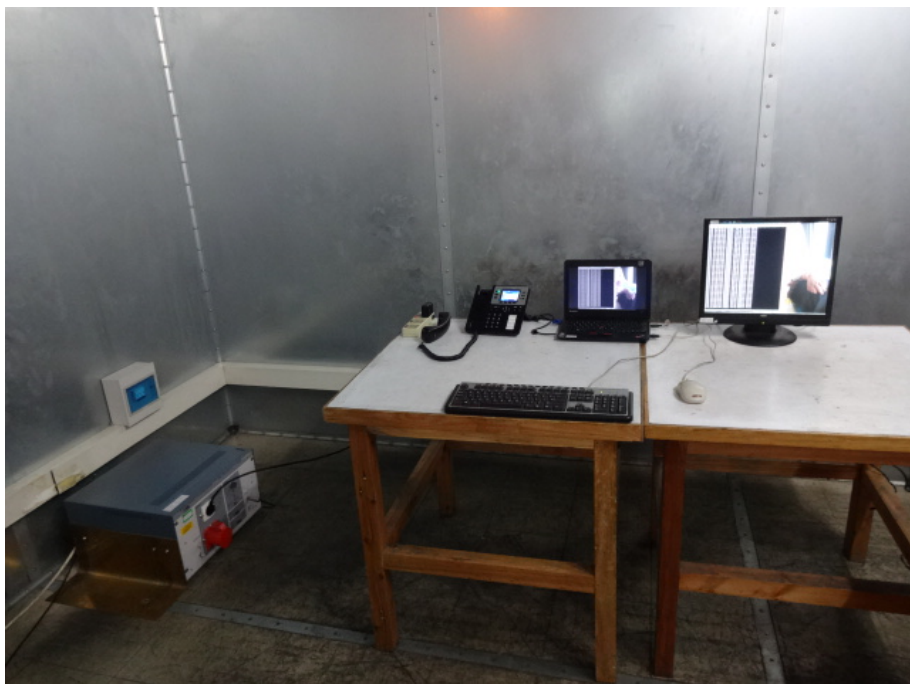
Conducted Emission Test Set-up -Front View
