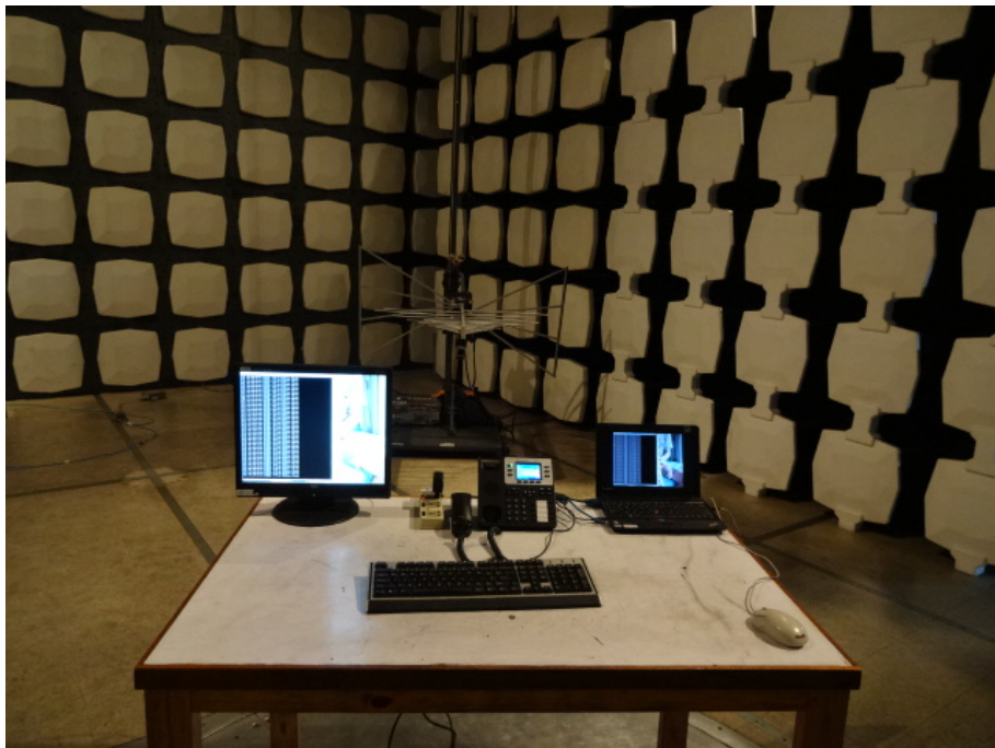
Radiated Emission Test Set-up (Below 1GHz)
