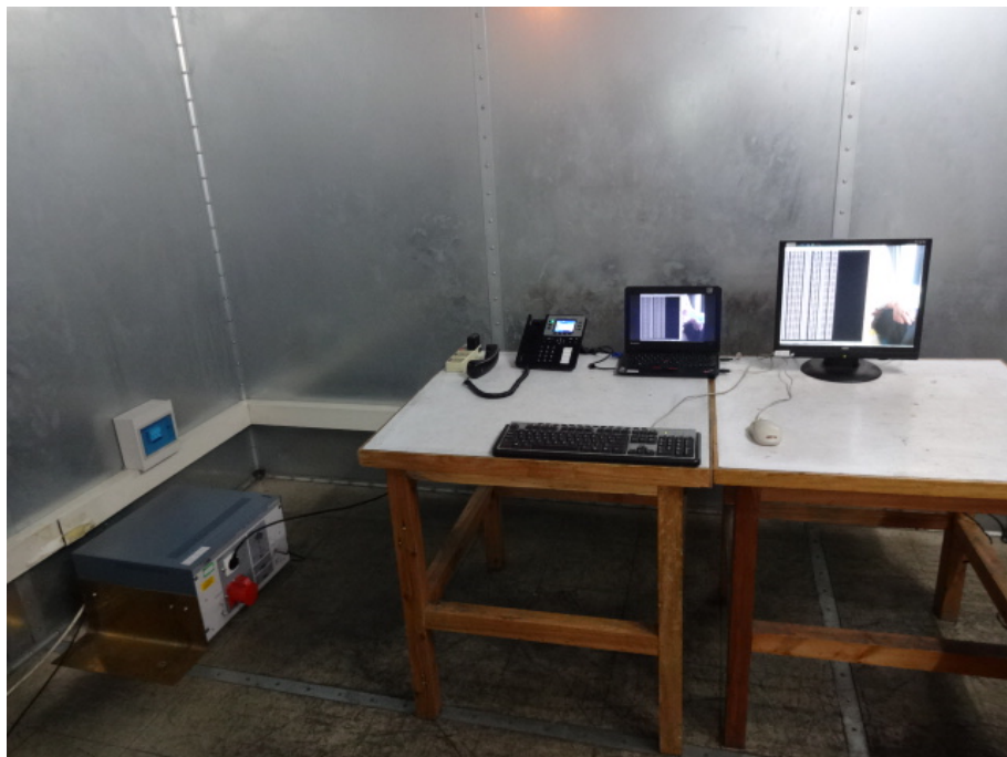
Conducted Emission Test Set-up -Front View
