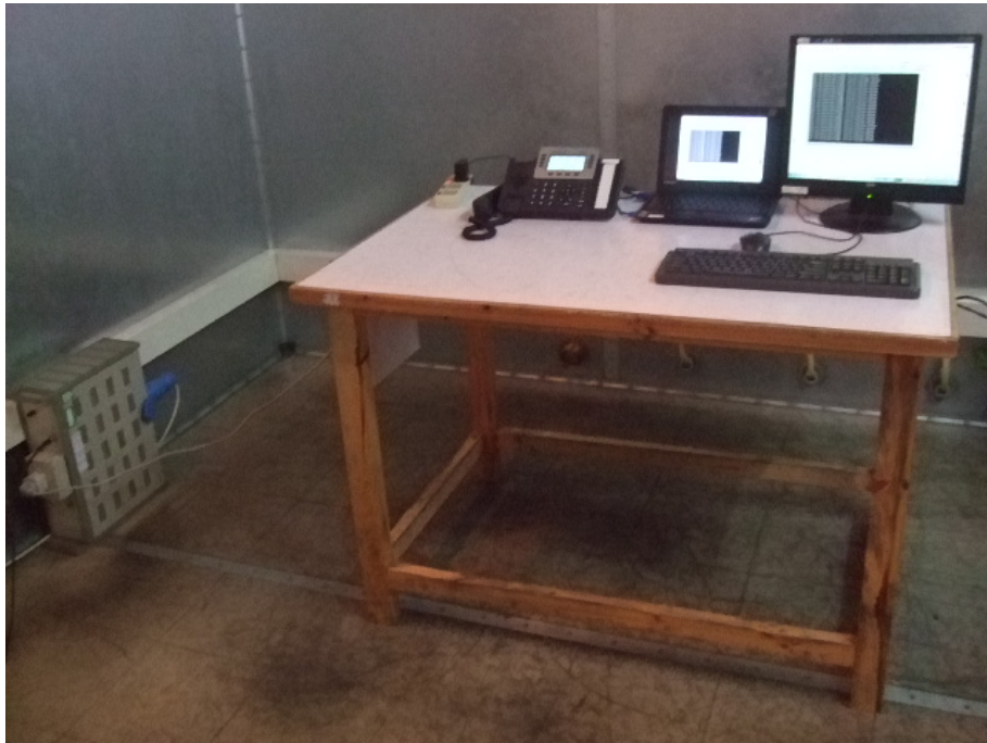
Conducted Emission Test Set-up
