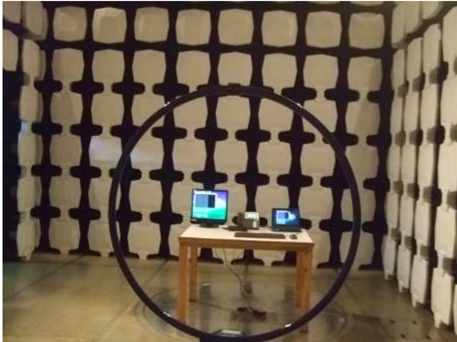
Radiated Emission Test Set-up (9KHz-30MHz)
