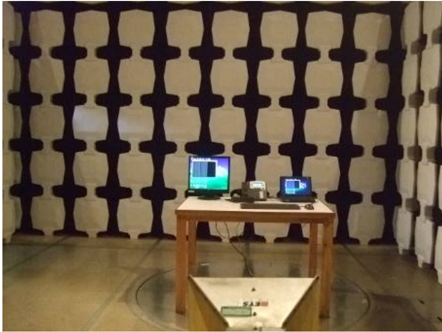
Radiated Emission Test Set-up (Above 1GHz)
