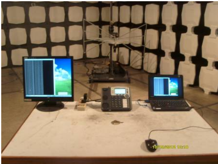
Radiated Emission Test Set-up (Below 1GHz)
