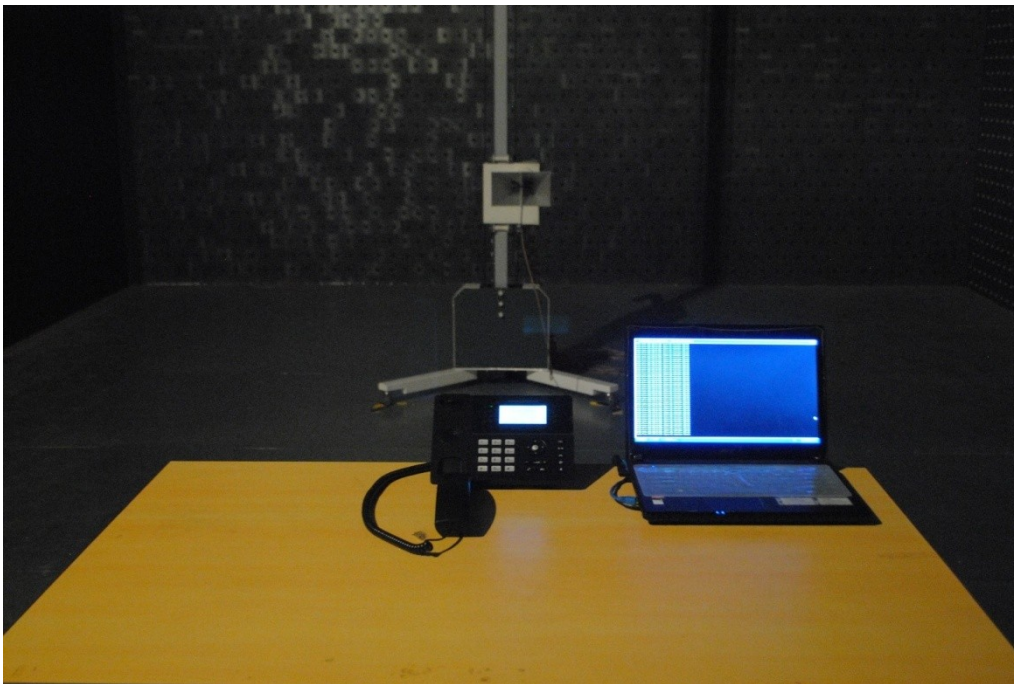
Radiated Emission test view (Frequency above 1GHz)
