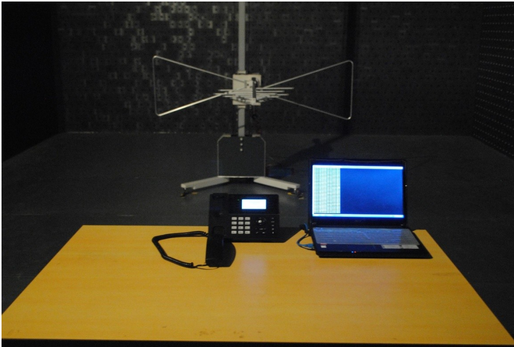
Radiated Emission test view (Frequency above 1GHz)
