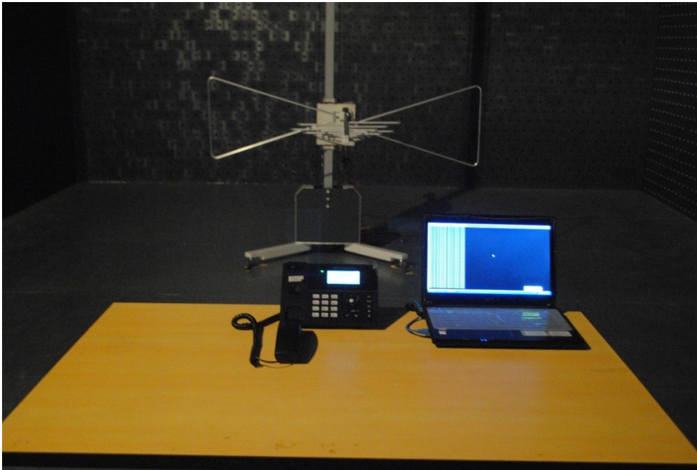
Radiated Emission test view (Frequency above 1GHz)
