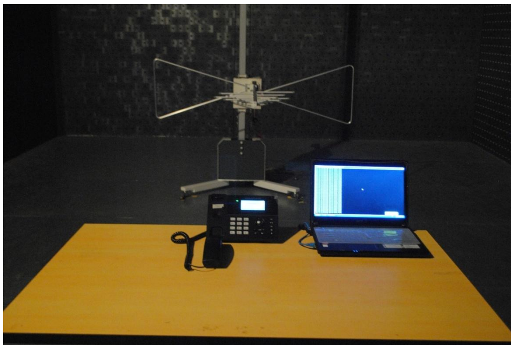
Radiated Emission test view (Frequency above 1GHz)
