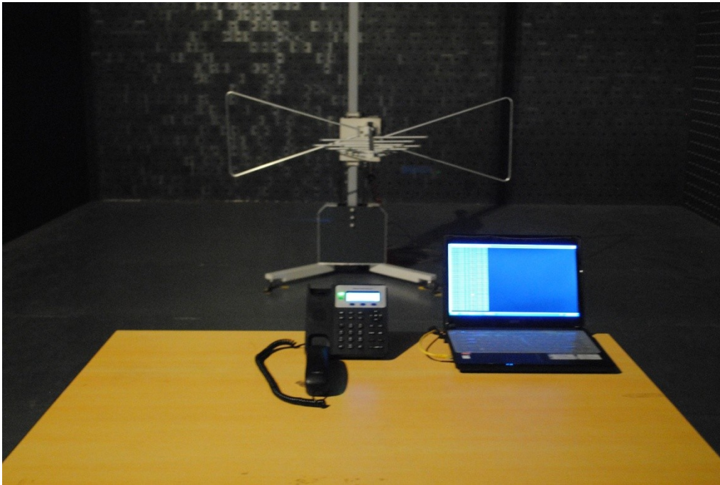
Radiated Emission test view (Frequency above 1GHz)
