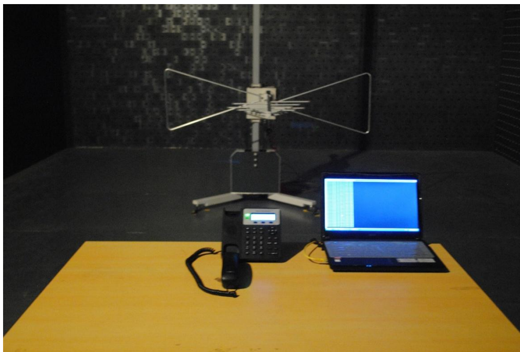
Radiated Emission test view (Frequency above 1GHz)
