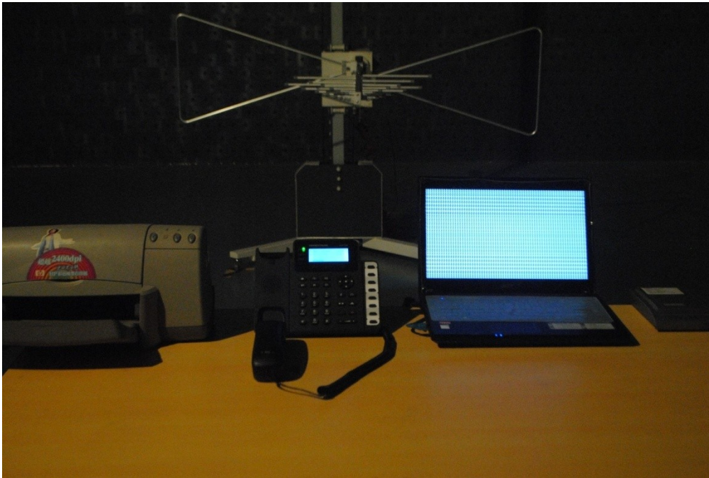
Radiated Emission test view (Frequency above 1GHz)
