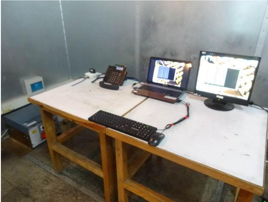
Conducted Emission Test Set-up -Front view
