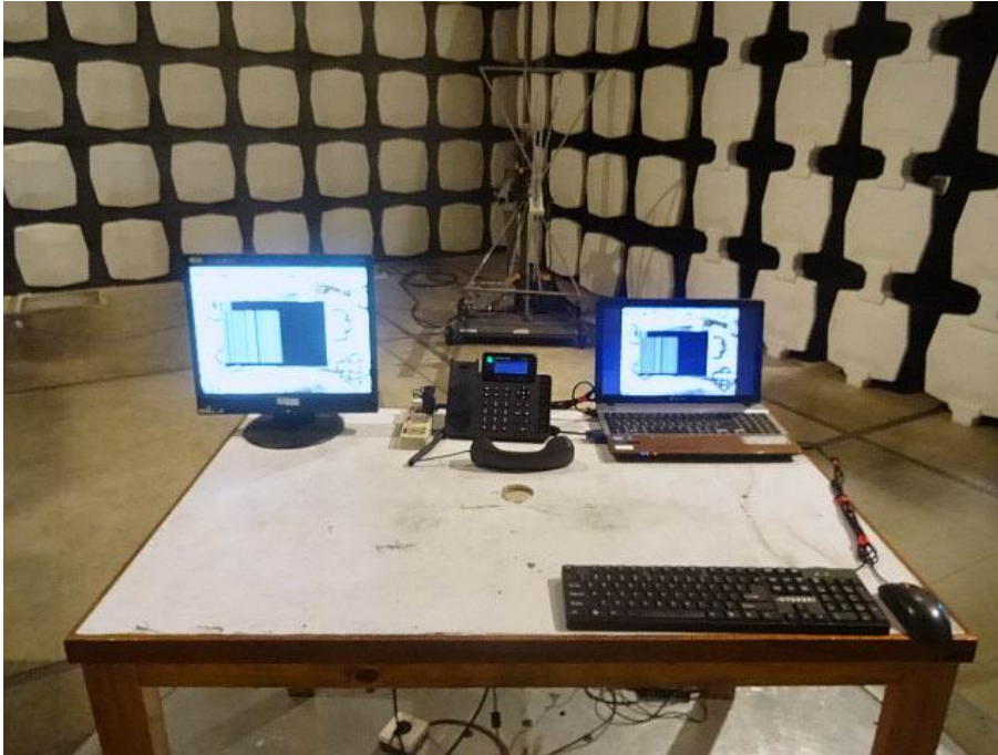
Radiated Emission Test Set-up(30-1000MHz)
