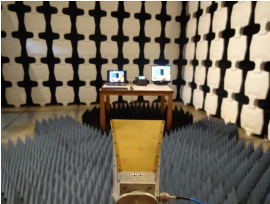
Radiated Emission Test Set-up(Above 1GHz)
