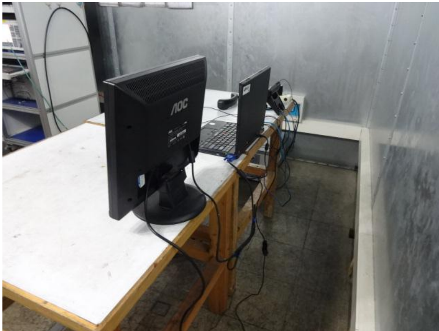
Conducted Emission Test Set-up –Rear View
