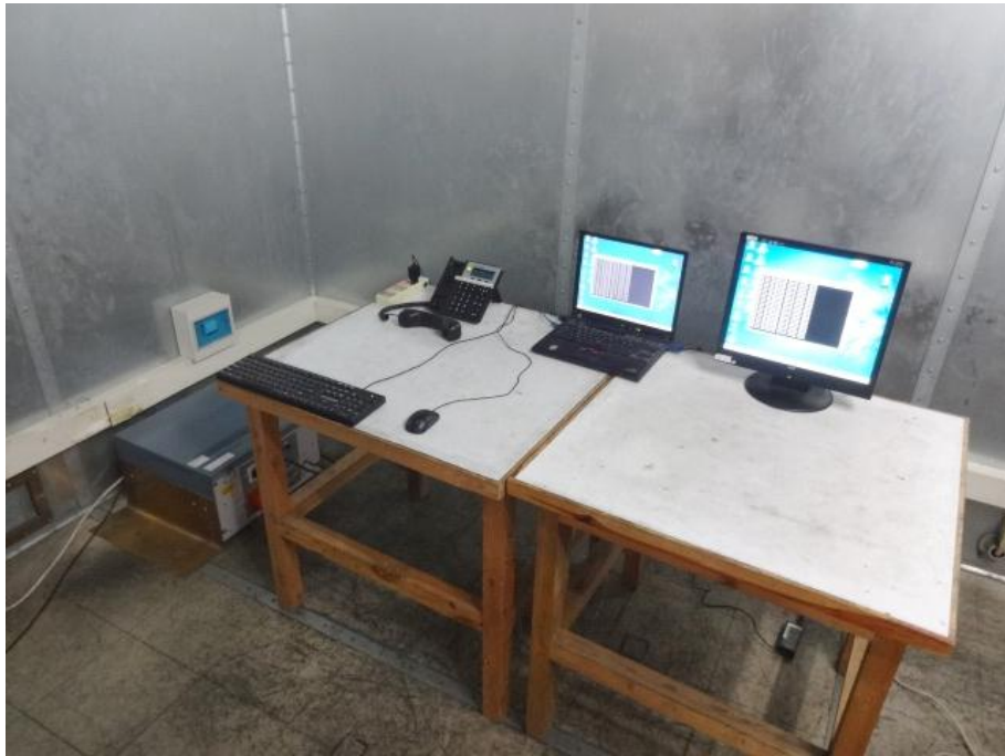
Conducted Emission Test Set-up –Front View
