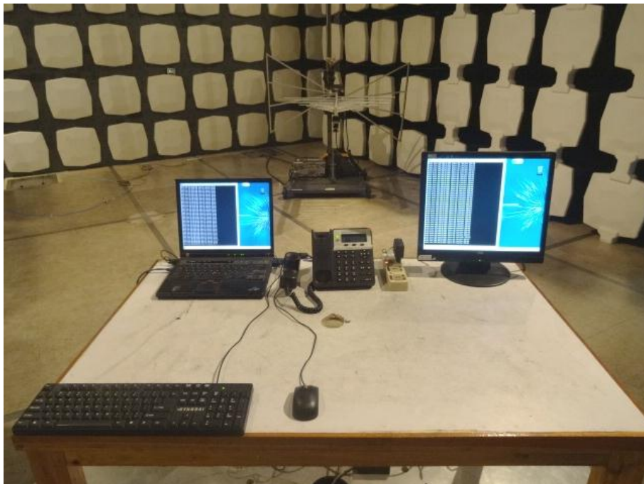
Radiated Emission Test Set-up (Below 1GHz)
