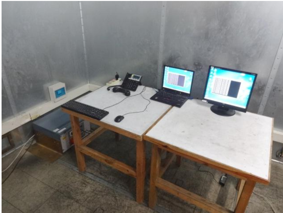
Conducted Emission Test Set-up -Front View
