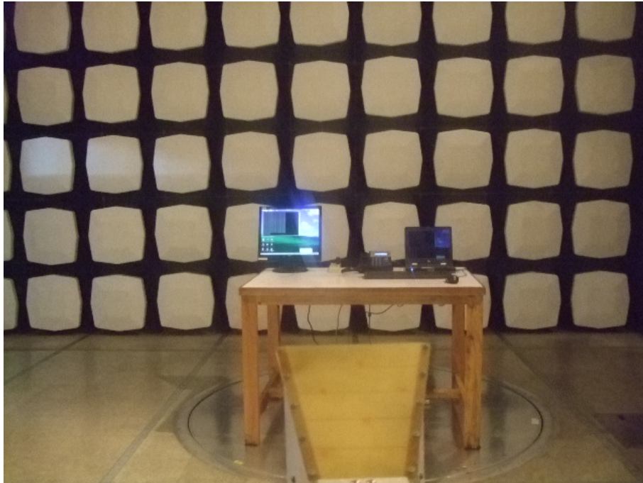
Radiated Emission Test Set-up(Above 1GHz)
