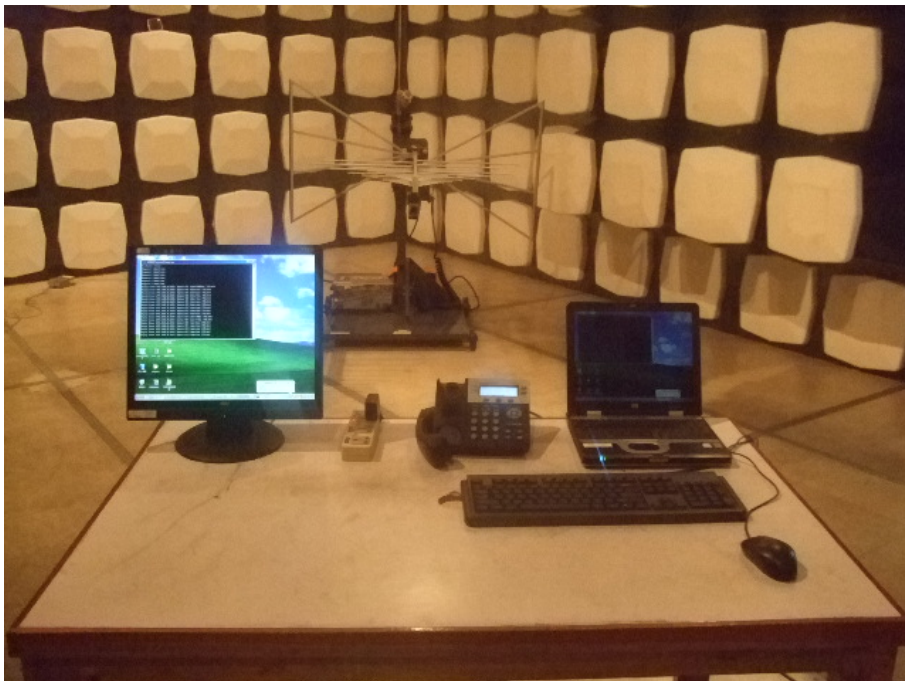
Radiated Emission Test Set-up(Below 1GHz)
