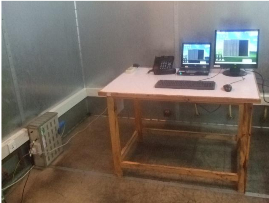
Conducted Emission Test Set-up
