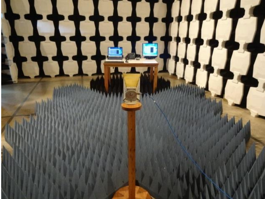
Radiated Emission Test Set-up (Above 1GHz)
