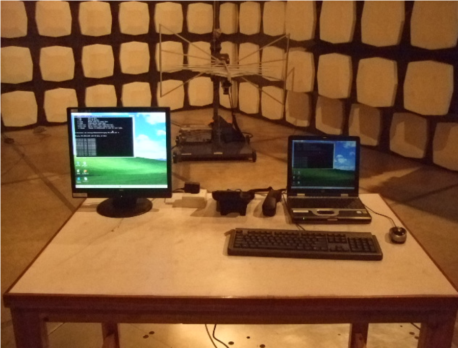
Radiated Emission Test Set-up(Below 1GHz)
