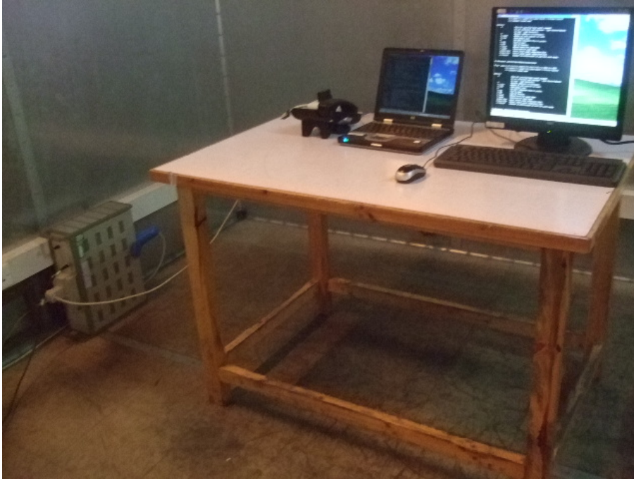
Conducted Emission Test Set-up -Connect to PC
