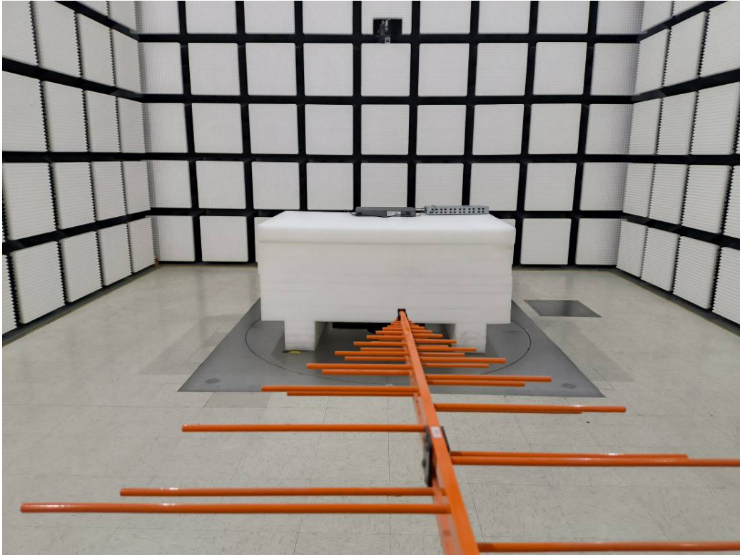
Radiated Emissions Below 1G Rear View-M1&M2
