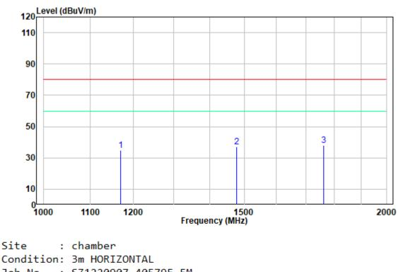
Condition: 3m HORIZONTAL Job No. : SZ1220907-40579E-EM Test Mode: System Operation With Full Load Note : RB150W01
