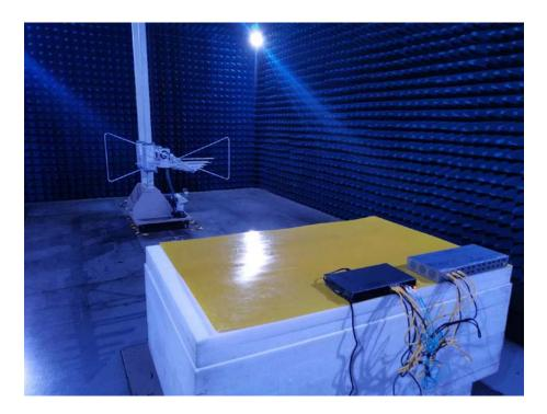
Photo of Radiated Emission Measurement (Above 1G) Test mode 1: System operation with Full load (G0970) Test mode 2: System operation with Full load (RB150W01) Test mode 3: System operation with Full load (BOF-150D54+12I)
