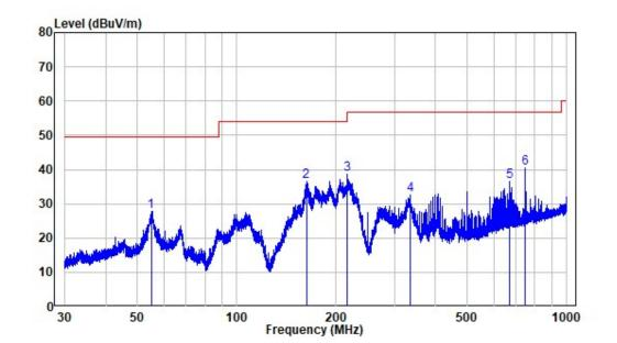
Site : chamber Condition: 3m HORIZONTAL Job No. : SZ1220907-40578E-EM Test Mode: System Operation With Full Load Note : R0001A(RB030W05-1202500)
