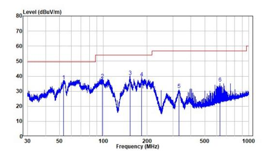
Site : chamber Condition: 3m VERTICAL Job No. : SZ1220907-40578E-EM Test Mode: System Operation With Full Load Note : R0001A(RB030W05-1202500)
