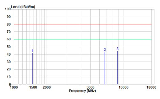
Site : chamber Condition: 3m Vertical Job No. : RA230426-22564E-EM Test Mode: System operation with Full load Note : BOU-45512-F
