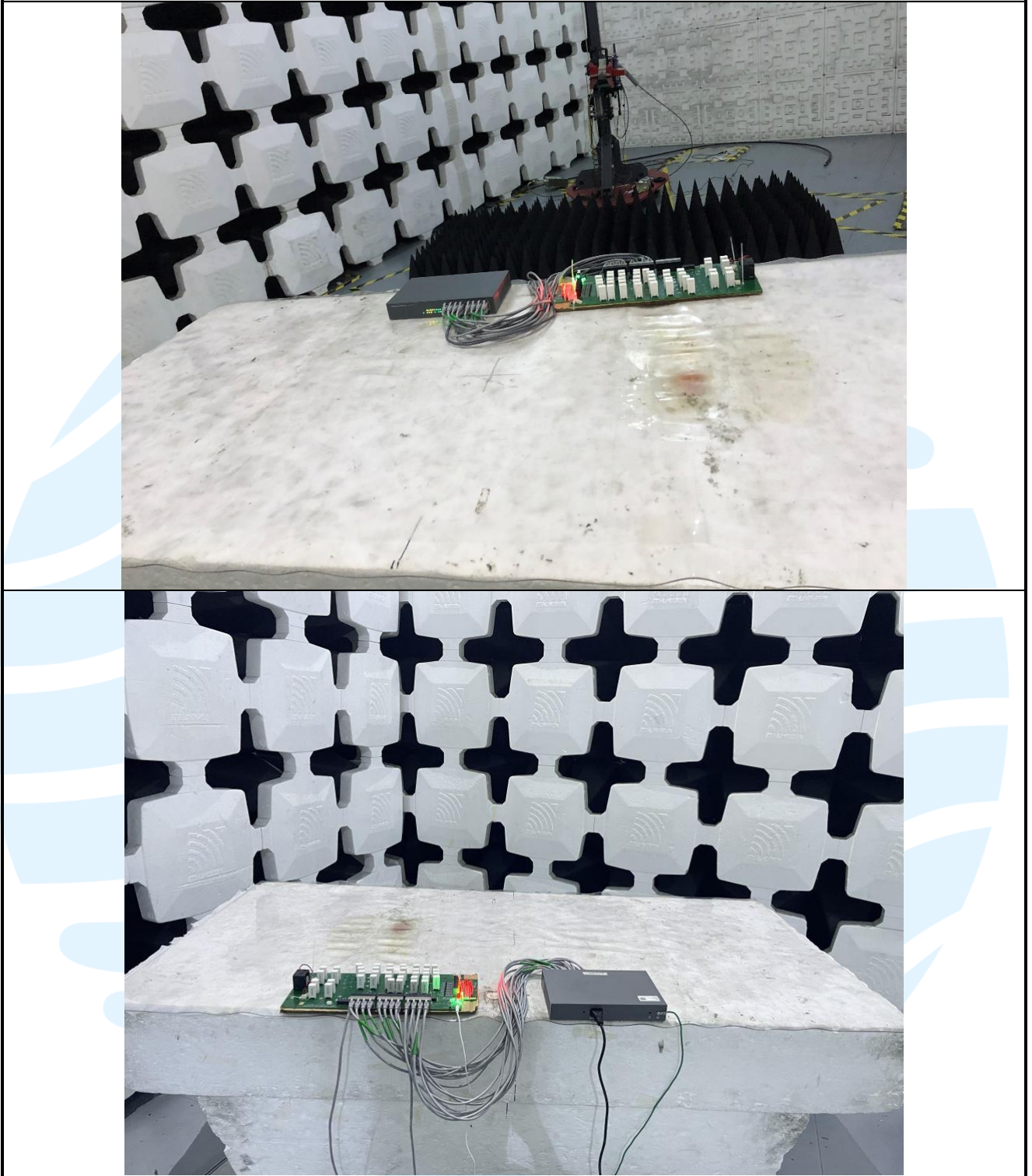
Radiated Emission Test Setup-2 (Above 1 GHz)
