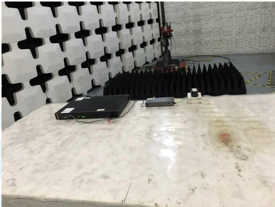
Radiated emission Test Setup-2 (Above 1 GHz)
