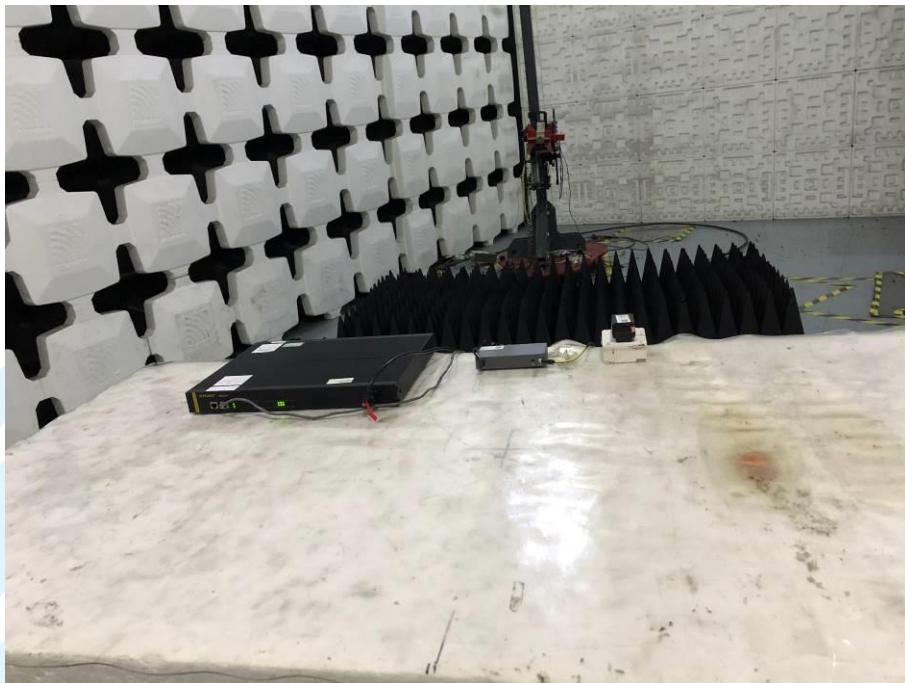
Radiated emission Test Setup-2 (Above 1 GHz)
