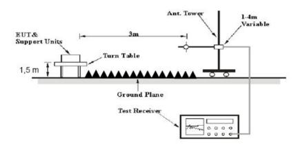
The radiated emissions were performed in the 3 meters distance, using the setup accordance with the ANSI C63.10-2013. The specification used was the FCC 15.209, and FCC 15.247, RSS-247, RSS-Gen limits.
