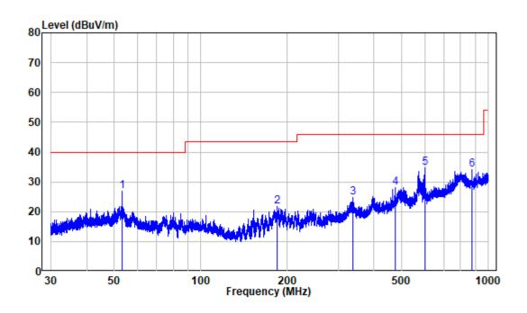
Site : chamber Condition: 3m VERTICAL Job No. : RA221230-64612E-RF Test Mode: Working
