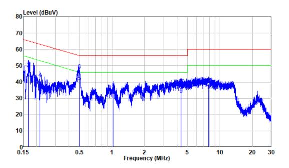
Site : Shielding Room Condition: Neutral EUT : Outdoor Long-Range Wi-Fi 6 Access Point M/N : GWN7660LR
