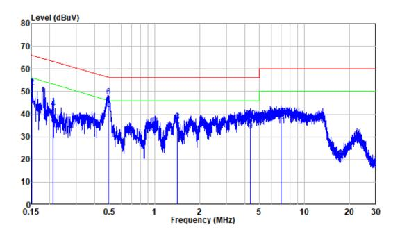
Site : Shielding Room Condition: Line EUT : Outdoor Long-Range Wi-Fi 6 Access Point M/N : GWN7660LR
