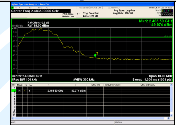
Out Of Band Emission 2LE_Channel 39
