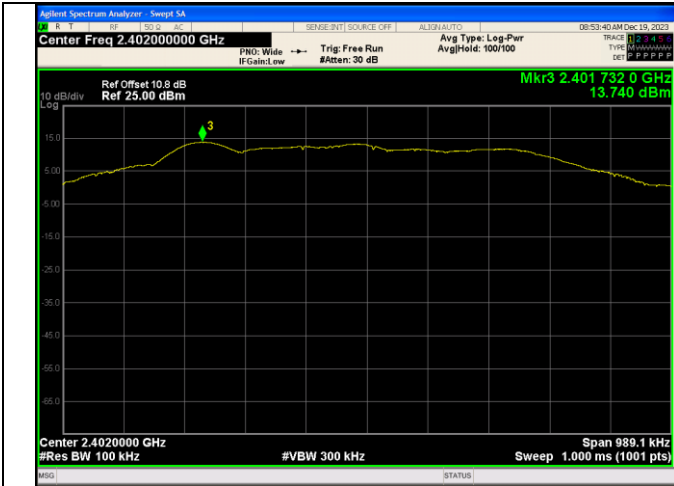
In-Band Reference Level LE Coded (S=2) Channel 0
