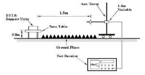
The radiated emission tests were performed in the 3 meters chamber, using the setup accordance with the ANSI C63.4-2014. The specification used was with the FCC Part 15 B Class B limits.
