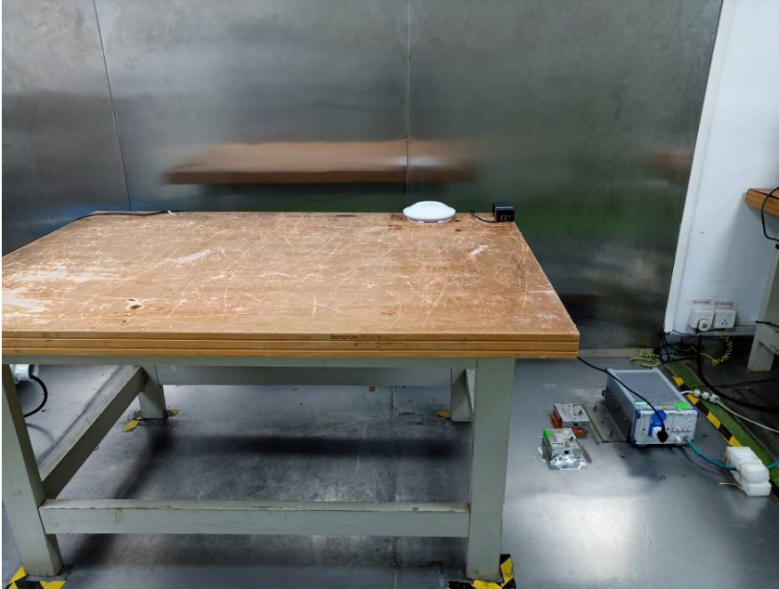
Conducted Emissions - Front View
