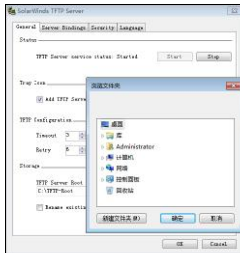
Figure 96 TFTP Server Directory Settings
