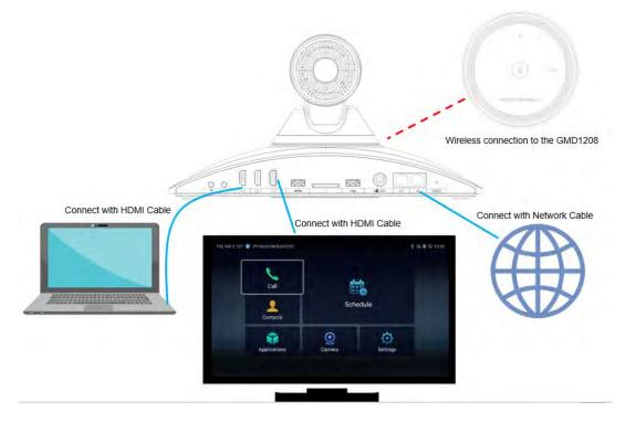
Figure 3: GVC3220 Back Panel Connection Diagram
