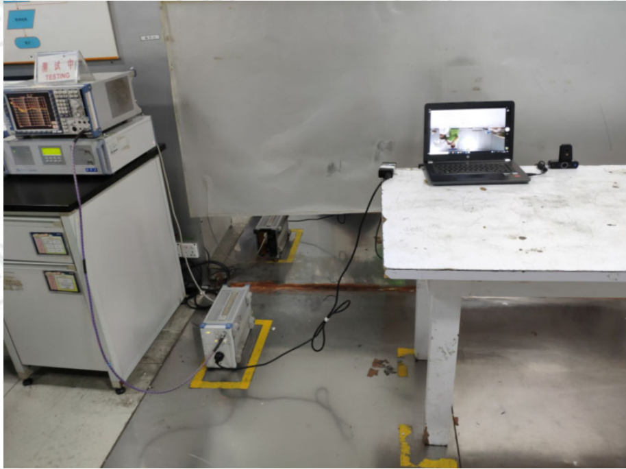
CONDUCTED DISTURBANCE TEST SETUP
