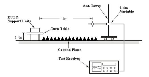
The radiated emission performed in the 3 meters, using the setup accordance with the ANSI C63.10-2013. The specification used was the FCC 15.209, FCC 15.247, RSS-247, RSS-Gen limits.
