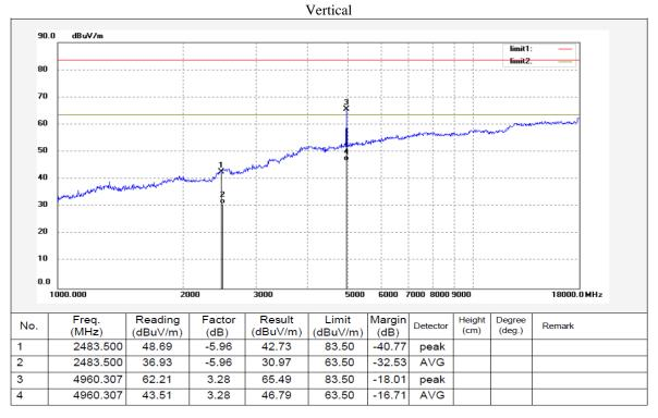
Note: Limit  $(dB\mu V/m)@1m = Limit (dB\mu V/m)@3m + 20log (3/1)$
