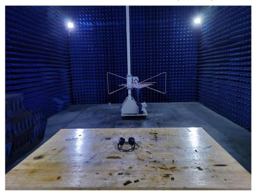
Photo of Radiated Emission Measurement (Above 1G)
