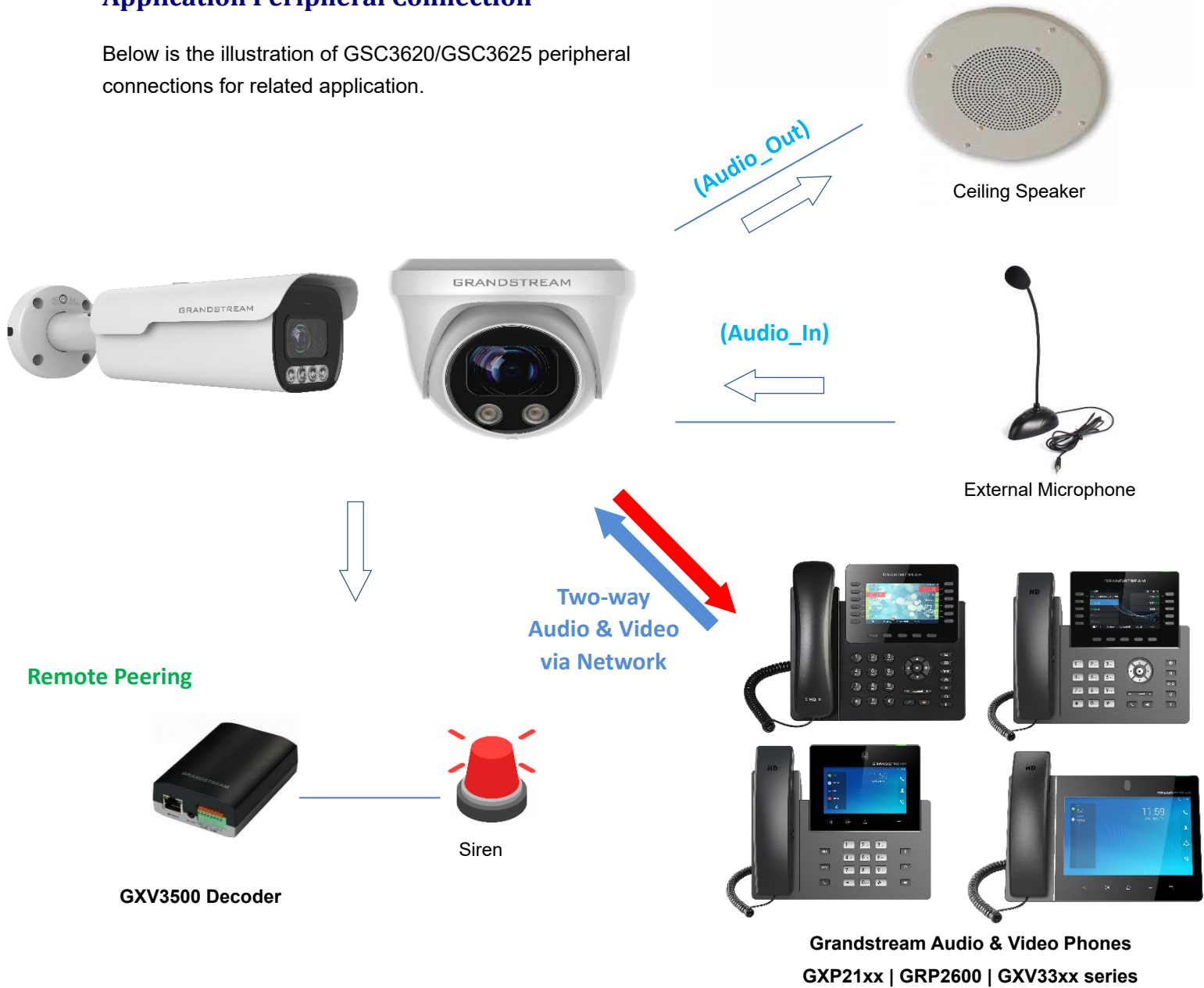
Figure 8: Application Peripheral Connection for GSC3620/GSC3625
