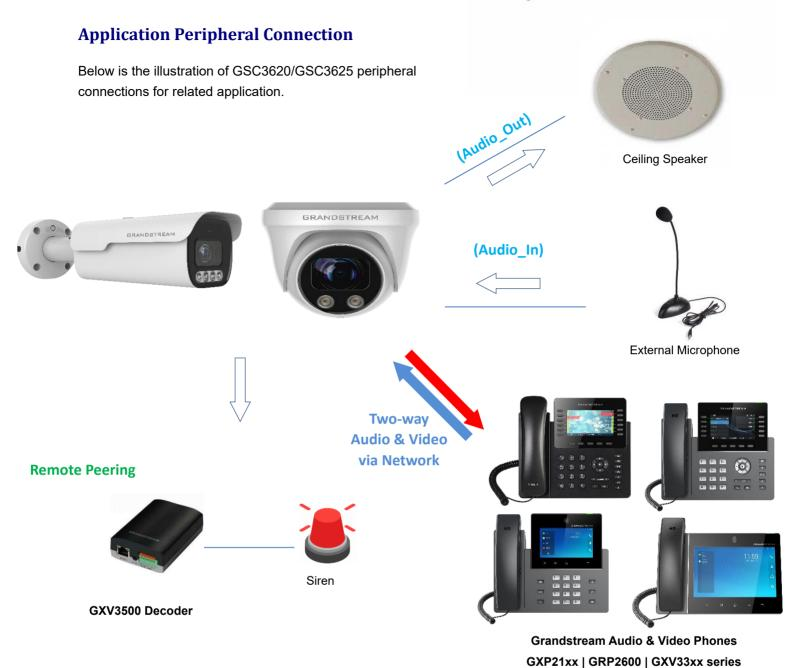
Figure 8: Application Peripheral Connection for GSC3620/GSC3625
