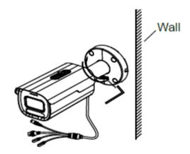
**Step 4:** Hold the body of camera and align to the notch as shown in the diagram, then push the body of camera into the cover of camera already mounted at the wall.
