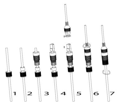
Figure 3: RJ45 plug installation
