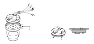
**Step 3:** Place the cable into the groove of camera cover, mount the cover into ceiling using provided screws as shown in below diagram. Leave the connectors of cable dangling outside the cover.
