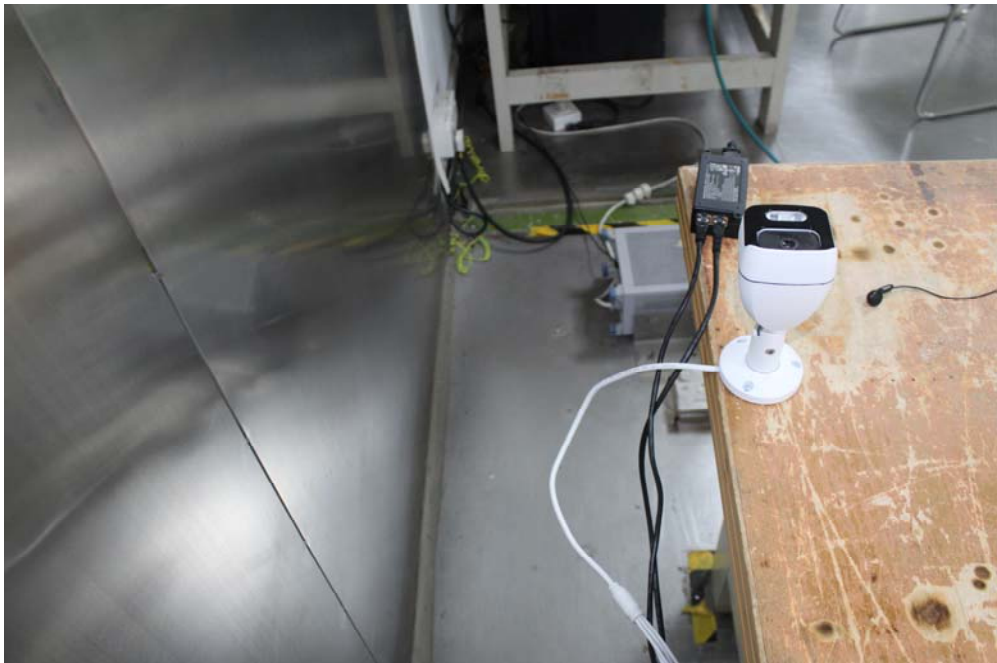
Conducted Emissions - Side View (For POE)
